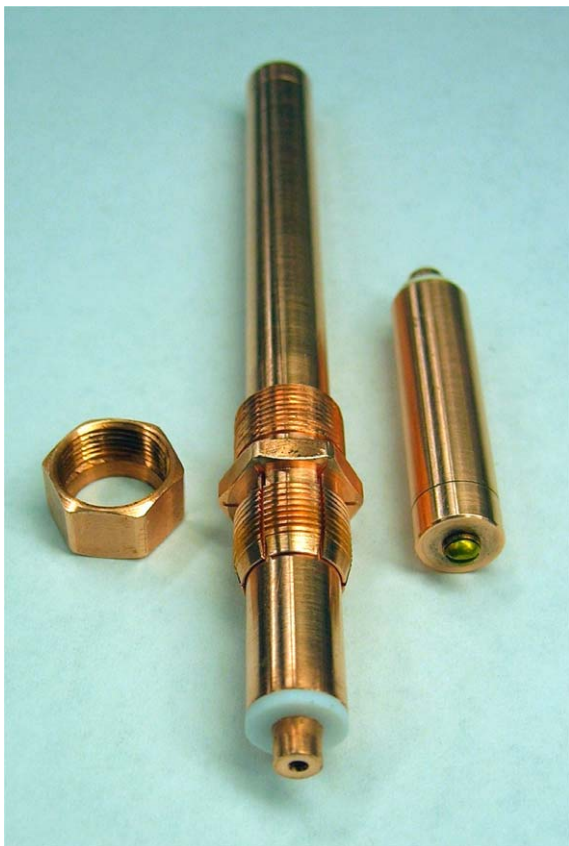
Fig. 3. A shorted coaxial trap of air dielectric is shown with a compression clamp that mounts it inside the probe. Another coaxial trap with a 99.9% \text{Al}_2\text{O}_3 dielectric is shown to the right.
